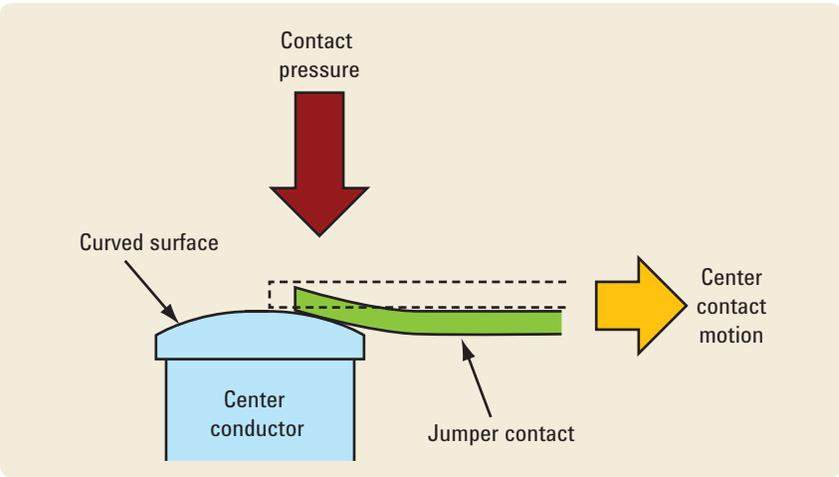
Figure 5. Electromechanical switch mating configuration illustrating microscopic wiping
