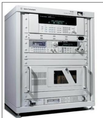
Figure 5: With LXI, a functional test system can fit into a rack that is just 400mm tall.
