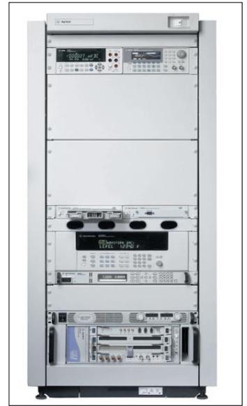
Figure 3: In an automotive test system, LXI components enable greater scalability and flexibility to meet test requirements.
