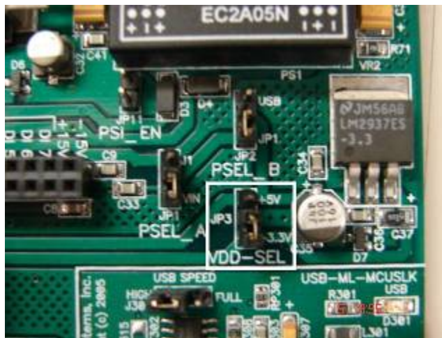
Figure 3. VDD_SEL Jumper on Project Board
