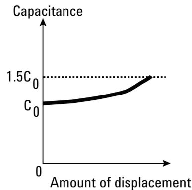
Figure 4. DC bias characteristic test for faster test throughput of capacitive sensors
