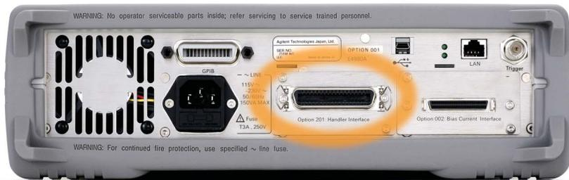
Figure 6. Agilent E4980A scanner interface
