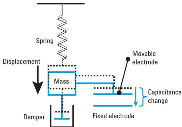
Figure 2. Principle operation of a MEMS capacitive sensor
