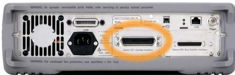
Figure 2. Agilent E4980A scanner interface
